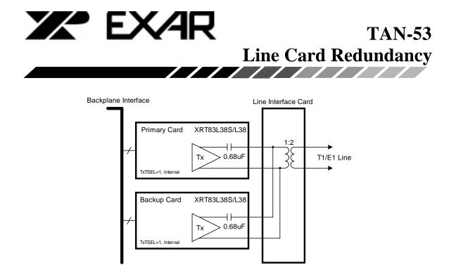
Figure 1b. Simplified Block Diagram of the Transmit Section for a 1:1 Redundancy Scheme Using One Common Transformer
