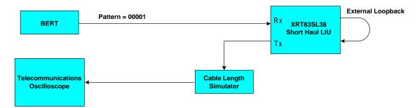
Figure 7 Simplified Lab Setup for Pulse Template Measurements
