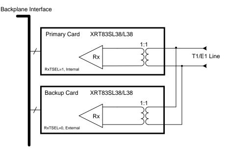
Figure 2a. Simplified Block Diagram of the Receive Section for a 1:1 Redundancy Scheme Using Two Transformers
