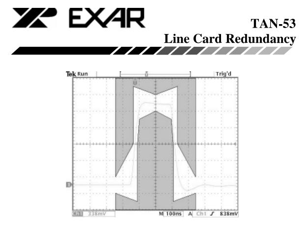
Figure 9 Pulse Template for E1 75ohm Impedance
