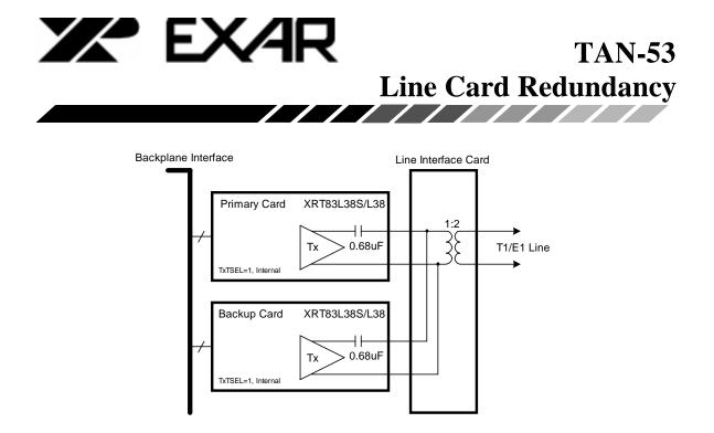
Figure 3b. Simplified Block Diagram of the Transmit Section for a 1+1 Redundancy Scheme Using One Common Transformer
