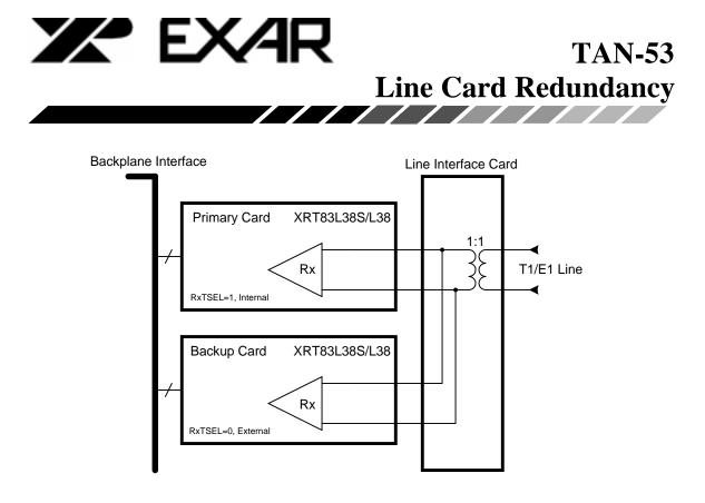
Figure 2b. Simplified Block Diagram of the Receive Section for a 1:1 Redundancy Scheme Using One Common Transformer
