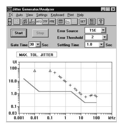
Figure 11 Jitter Tolerance for E1 75ohm
