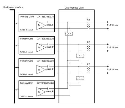
Figure 5. Simplified Block Diagram of the Transmit Section for an N+1 Redundancy Scheme
